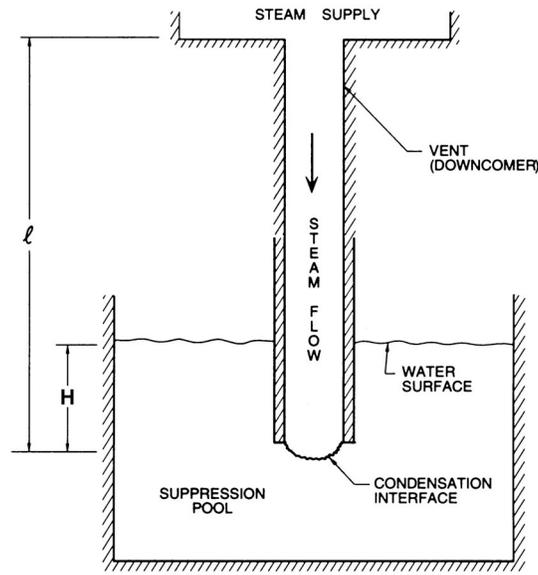
Figure 1: Components of a pressure suppression system.
