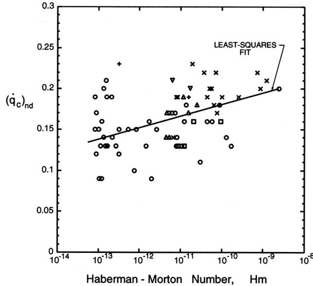
Figure 3: Data on the dimensionless critical heat flux,  $(\dot{q}_c)_{nd}$  (or  $C_2$ ), plotted against the Haberman-Morton number,  $Hm = g\mu_L^4(1 - \rho_V/\rho_L)/\rho_L S^3$ , for water (+), pentane ( $\times$ ), ethanol ( $\square$ ), benzene ( $\triangle$ ), heptane ( $\nabla$ ) and propane ( $*$ ) at various pressures and temperatures. Adapted from Borishanski (1956) and Zuber *et al.* (1961).
