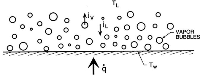
Figure 1: Nucleate boiling.
