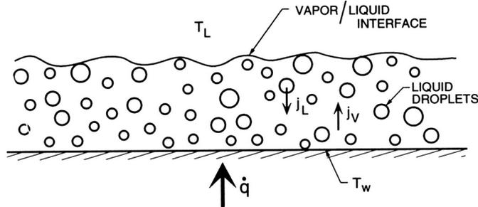
Figure 2: Sketch of the conditions close to film boiling.
