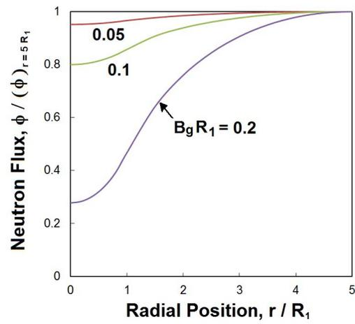
Figure 3: Typical neutron flux profiles for the control rod lattice cell with  $R_2/R_1 = 5$  for three values of non-dimensional geometric buckling,  $B_g R_1$ , as shown.
