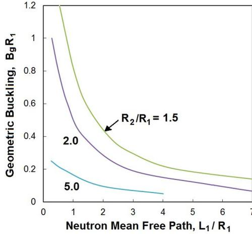
Figure 2: Values of the non-dimensional geometric buckling for the control rod lattice cell as a function of  $L_1/R_1$  for three values of  $R_2/R_1$  as shown.
