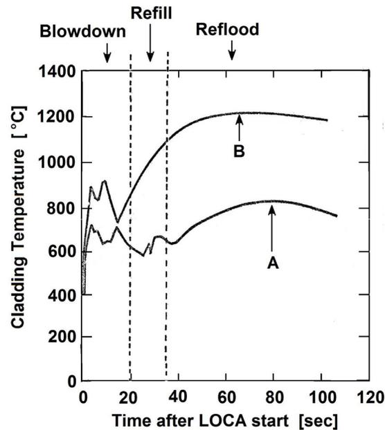
Figure 1: Estimated maximum temperature in the cladding during a postulated LOCA in a PWR as a function of time: (A) using realistic assumptions and (B) using conservative assumptions. Adapted from Hsu (1978).
