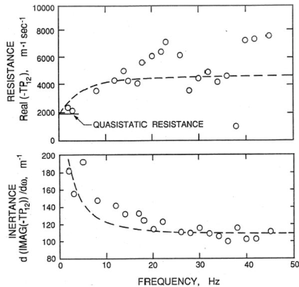
Figure 2: Typical inertia and resistance values from the centrifugal pump data of figure 1. Data do not include the diffuser contribution. The lines correspond to analytical values obtained as described in the text.
