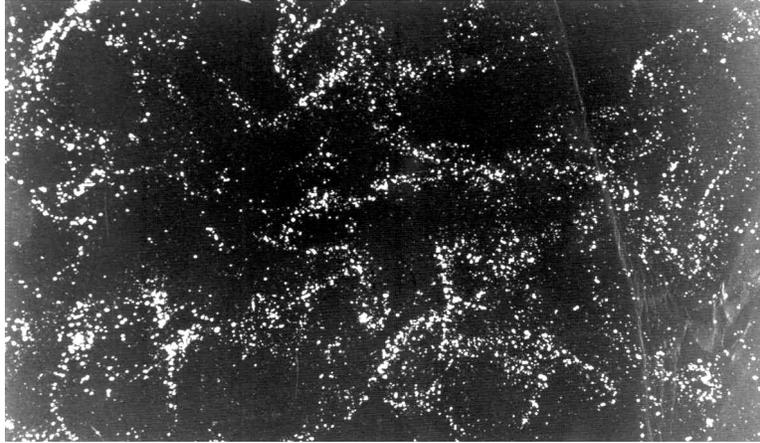
Figure 3: Image of the centerplane of a fully developed, turbulent channel flow of air loaded with  $28\mu\text{m}$  particles. The area is  $50\text{mm}$  by  $30\text{mm}$ . Reproduced from Fessler *et al.*(1994) with the authors' permission.
