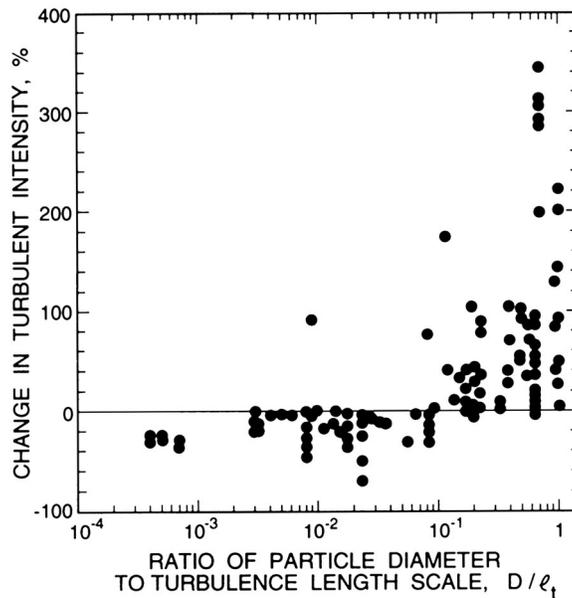
Figure 1: The percentage change in the turbulence intensity as a function of the ratio of particle size to turbulence length scale,  $D/\ell_t$ , from a wide range of experiments. Adapted from Gore and Crowe (1989).
