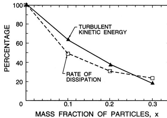
Figure 2: The percentage change in the turbulent kinetic energy and the rate of viscous dissipation with mass fraction for a channel flow of  $150\mu\text{m}$  glass spheres suspended in air (from Paris and Eaton 2001).
