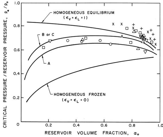
Figure 2: The ratio of critical pressure,  $p_*$ , to reservoir pressure,  $p_o$ , plotted against the reservoir vapor volume fraction,  $\alpha_o$ , for water/steam mixtures. The data and the partially frozen model results are for the same conditions as in figure 1.
