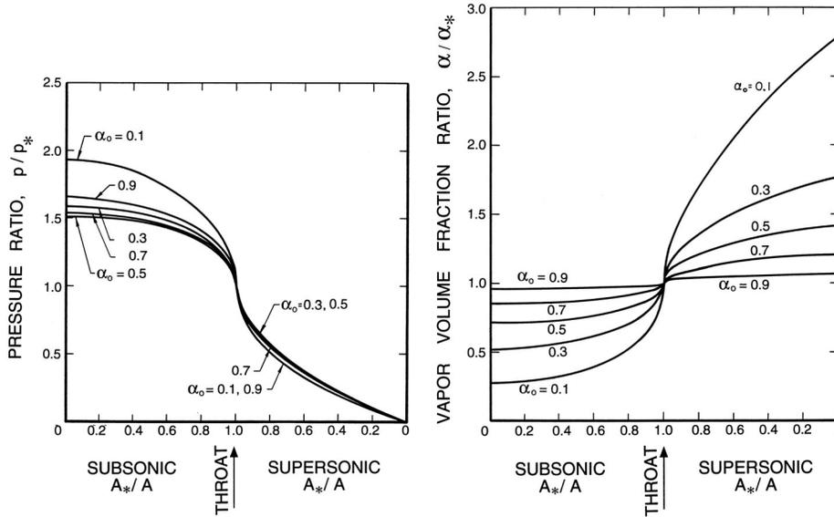
Figure 3: Left: Ratio of the pressure,  $p$ , to the critical pressure,  $p_*$ , and Right: Ratio of the vapor volume fraction,  $\alpha$ , to the critical vapor volume fraction,  $\alpha_*$ , as functions of the area ratio,  $A_*/A$ , for the case of water with  $g^* = 1.67$ ,  $\eta = 0.73$ ,  $g_V = 0.91$ , and  $f_V = 0.769$ .
