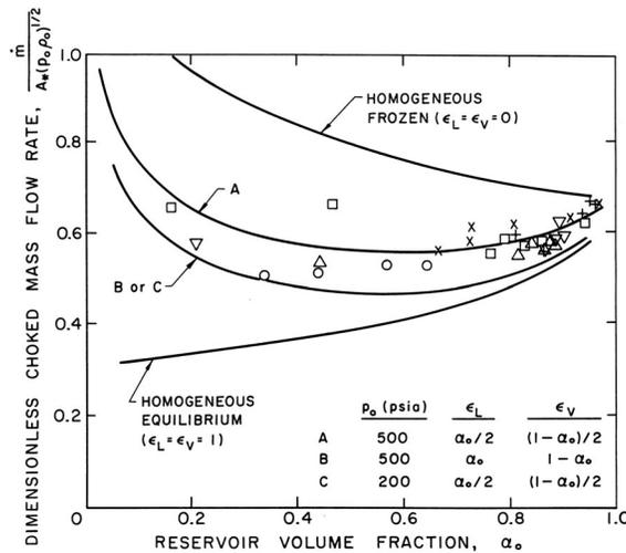
Figure 1: The dimensionless choked mass flow rate,  $\dot{m}/A_*(p_o \rho_o)^{1/2}$ , plotted against the reservoir vapor volume fraction,  $\alpha_o$ , for water/steam mixtures. The data shown is from the experiments of Maneely (1962) and Neusen (1962) for 100 → 200 psia (+), 200 → 300 psia (×), 300 → 400 psia (□), 400 → 500 psia (△), 500 → 600 psia (▽) and > 600 psia (\*). The theoretical lines use  $g^* = 1.67$ ,  $\eta = 0.73$ ,  $g_V = 0.91$ , and  $f_V = 0.769$  for water.
