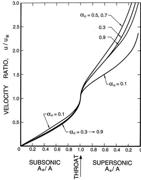
Figure 4: Ratio of the velocity,  $u$ , to the critical velocity,  $u_*$ , as a function of the area ratio for the same case as figure 3.
