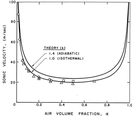
Figure 2: The sonic velocity in a bubbly air/water mixture at atmospheric pressure for  $k = 1.0$  and  $1.4$ . Experimental data presented is from Karplus (1958) and Gouse and Brown (1964) for frequencies of  $1 \text{ kHz}$  ( $\odot$ ),  $0.5 \text{ kHz}$  ( $\square$ ), and extrapolated to zero frequency ( $\triangle$ ).
