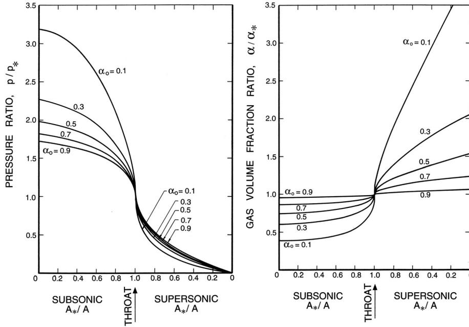
Figure 3: Left: Ratio of the pressure,  $p$ , to the throat pressure,  $p_*$ , and Right: Ratio of the void fraction,  $\alpha$ , to the throat void fraction,  $\alpha_*$ , for two-component flow in a duct with isothermal gas behavior.
