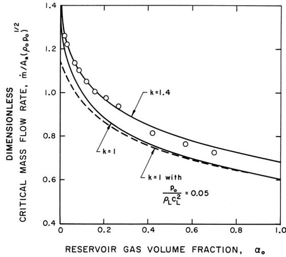
Figure 2: Dimensionless critical mass flow rate,  $\dot{m}/A_*(p_o \rho_o)^{1/2}$ , as a function of  $\alpha_o$  for choked flow of a gas/liquid flow through a nozzle. Solid lines are incompressible liquid results for polytropic indices of 1.4 and 1.0. Dashed line shows effect of liquid compressibility for  $p_o/\rho_L c_L^2 = 0.05$ . The experimental data ( $\odot$ ) are from Muir and Eichhorn (1963).
