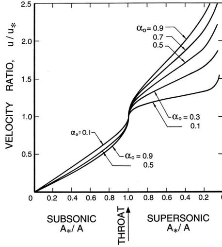
Figure 4: Ratio of the velocity,  $u$ , to the throat velocity,  $u_*$ , for two-component flow in a duct with isothermal gas behavior.
