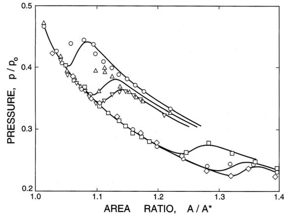
Figure 2: Experimental pressure profiles through condensation *fronts* in a diffuser for six different initial conditions. Also shown are the corresponding theoretical results. From Binnie and Green (1942) and Hill (1966).
