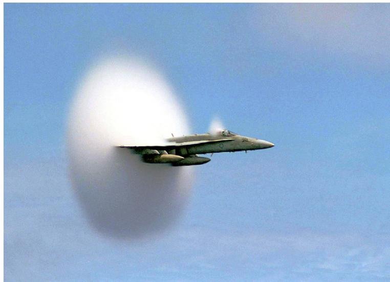
Figure 3: Condensation *fronts* in the flow around a transonic F/A-18 Hornet operating in humid conditions. U.S. Navy photograph by Ensign John Gay.
