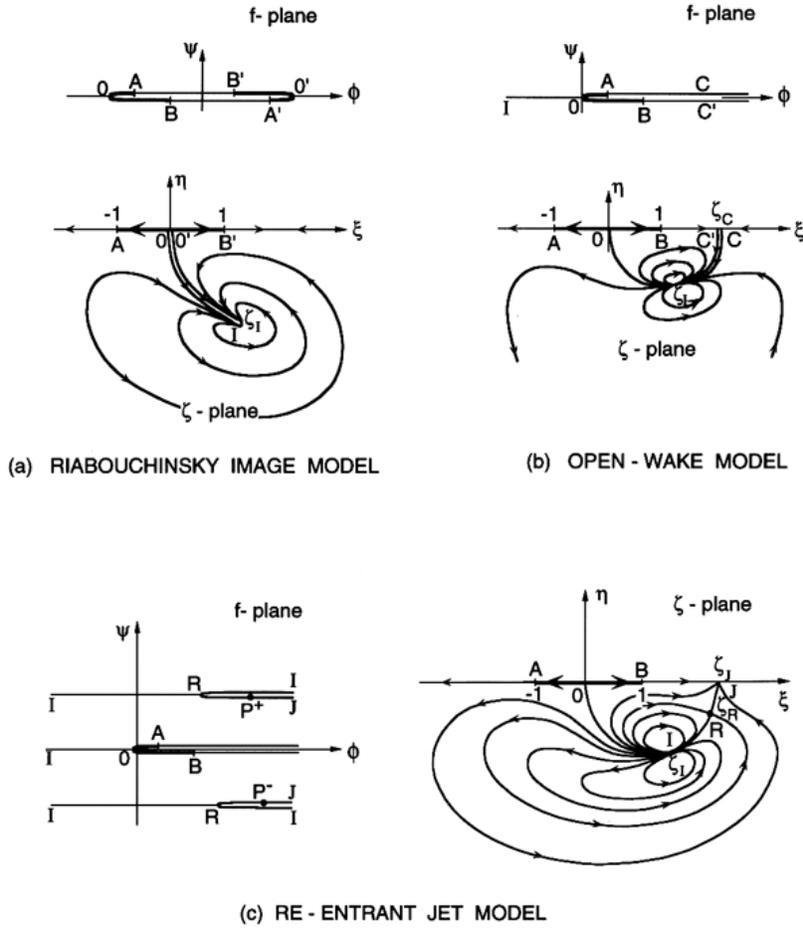
Figure 1: Streamlines in the complex potential  $f$ -plane and the parametric  $\zeta$ -plane where the flow boundaries and points correspond to those of section (Nub).
