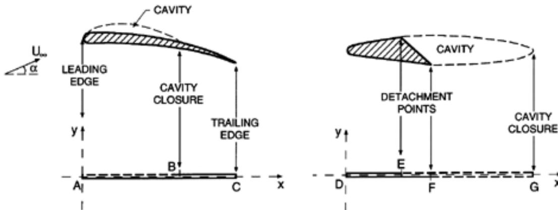
Figure 1: Examples of the linearized geometry (lower figures) for two planar cavity flows (upper sketches): a partially cavitating foil (left) and a supercavitating headform (right). Solid boundaries are indicated by the thick lines and the free streamlines by the thick dashed lines.
