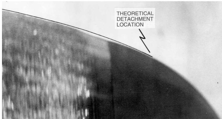
Figure 4: Comparison of the theoretical and experimental profiles of a fully developed cavity behind a sphere. The flow is from the right to the left. From Brennen (1969a).
