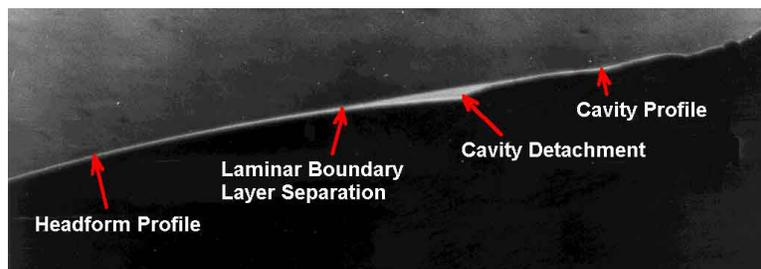
Figure 6: Schlieren photograph showing boundary layer separation upstream of the free surface detachment on an axisymmetric headform. The cavitation number is 0.39 and the tunnel velocity is  $8.1 \text{ m/s}$ . The actual distance between the separation and detachment points is about  $0.28 \text{ cm}$ . Reproduced from Arakeri (1975) with permission of the author.
