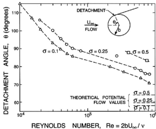
Figure 3: Observed free surface detachment points from spheres for various cavitation numbers,  $\sigma$ , and Reynolds numbers. Also shown are the potential flow values using the smooth detachment condition. Adapted from Brennen (1969b).
