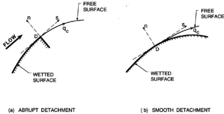
Figure 1: Notation used in the discussion of the detachment of a free streamline from a solid body.
