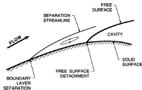
Figure 5: Model of the flow in the vicinity of a smooth detachment point. Adapted from Arakeri (1975).
