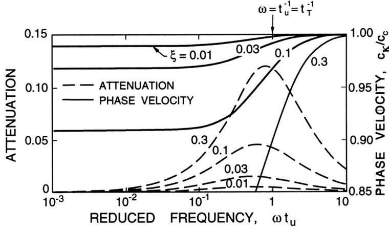
Figure 1: Non-dimensional attenuation,  $Im\{-\kappa c_C/\omega\}$  (dotted lines), and phase velocity,  $c_\kappa/c_C$  (solid lines), as functions of reduced frequency,  $\omega t_u$ , for a dusty gas with various loadings,  $\xi$ , as shown and  $\gamma = 1.4$ ,  $t_T/t_u = 1$  and  $c_{pC}/c_{sD} = 0.3$ .
