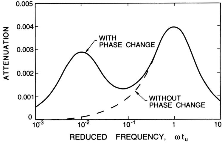
Figure 3: Non-dimensional attenuation,  $Im\{-\kappa c_C/\omega\}$ , as a function of reduced frequency for a droplet-laden gas flow with  $\xi = 0.01$ ,  $\gamma = 1.4$ ,  $t_T/t_u = 1$  and  $c_{pC}/c_{sD} = 1$ . The dashed line is the result without phase change; the solid line is an example of the alteration caused by phase change. Adapted from Marble and Wooten (1970).
