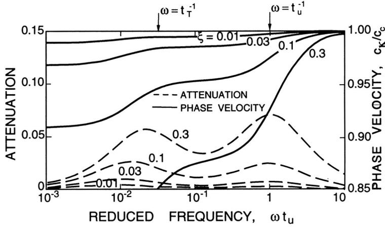
Figure 2: Non-dimensional attenuation,  $Im\{-\kappa c_C/\omega\}$  (dotted lines), and phase velocity,  $c_\kappa/c_C$  (solid lines), as functions of reduced frequency,  $\omega t_u$ , for a dusty gas with various loadings,  $\xi$ , as shown and  $\gamma = 1.4$ ,  $t_T/t_u = 30$  and  $c_{pC}/c_{sD} = 0.3$ .
