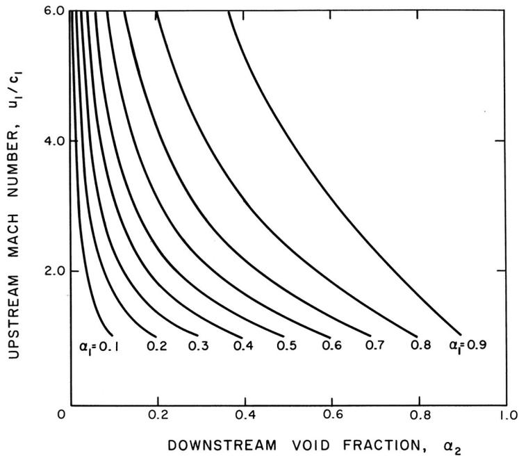
Figure 3: The upstream Mach number,  $u_1/c_1$ , as a function of the upstream and downstream void fractions,  $\alpha_1$  and  $\alpha_2$ , for  $k = 1.4$  and  $R_1(p_1 - p_V)/S = 200$ .
