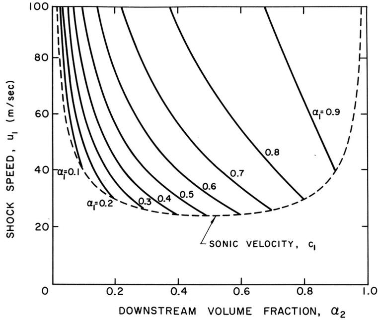
Figure 2: Shock speed,  $u_1$ , as a function of the upstream and downstream void fractions,  $\alpha_1$  and  $\alpha_2$ , for the particular case  $(p_1 - p_V)/\rho_L = 100 \text{ m}^2/\text{sec}^2$ ,  $2S/\rho_L R_1 = 0.1 \text{ m}^2/\text{sec}^2$ , and  $k = 1.4$ . Also shown by the dotted line is the sonic velocity,  $c_1$ , under the same upstream conditions.
