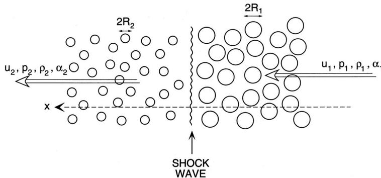
Figure 1: Schematic of the flow relative to a bubbly shock wave.
