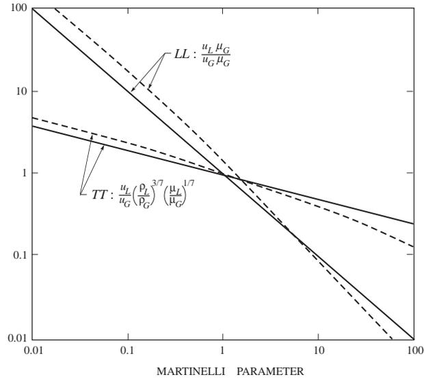
Figure 4: Ratios demonstrating the velocity ratio,  $u_L/u_G$ , implicit in the Lockhart-Martinelli correlation as functions of the Martinelli parameter,  $Ma$ , for the  $LL$  and  $TT$  cases. Solid lines:  $\kappa_L = \kappa_G = 1$ ; dashed lines:  $\kappa_L = 1/(1 - \alpha)$ ,  $\kappa_G = 1$ .
