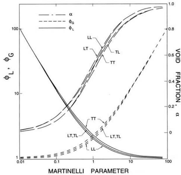
Figure 1: The Lockhart-Martinelli correlation results for  $\phi_L$  and  $\phi_G$  and the void fraction,  $\alpha$ , as functions of the Martinelli parameter,  $Ma$ , for the case,  $\kappa_L = \kappa_G = 1$ . Results are shown for the four laminar and turbulent stream permutations,  $LL$ ,  $LT$ ,  $TL$  and  $TT$ .
