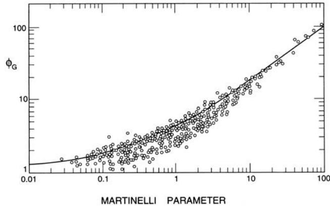
Figure 3: Comparison of the Lockhart-Martinelli correlation (the  $TT$  case) for  $\phi_G$  (solid line) with experimental data. Adapted from Turner and Wallis (1965).
