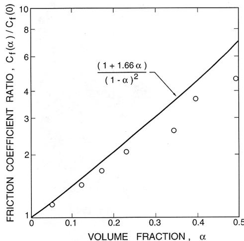
Figure 1: The ratio of the *base curve* friction coefficient at finite loading,  $C_f(\alpha)$ , to the friction coefficient for the continuous phase alone,  $C_f(0)$ . Equation ?? (line) is compared with the data of Lazarus and Neilsen (1978).
