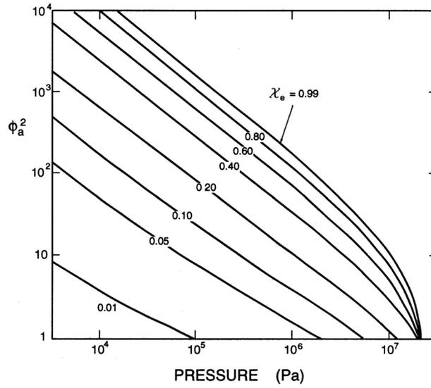
Figure 3: The Martinelli-Nelson acceleration pressure drop function,  $\phi_a^2$ , for water as a function of the prevailing pressure level and the exit mass quality,  $\mathcal{X}_e$ . Case shown is for  $\kappa_L = \kappa_G = 1.0$  and  $m_L = m_G = 0.25$ .
