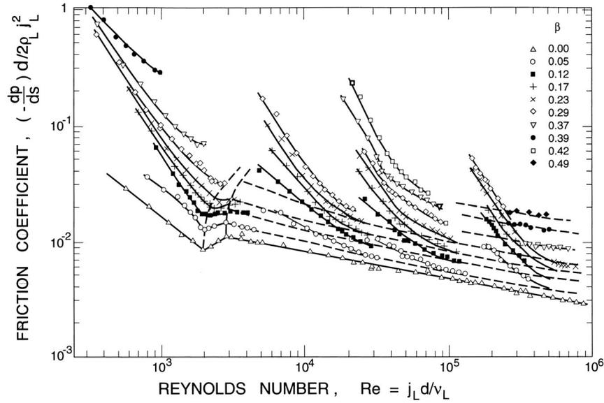
Figure 2: Typical friction coefficients (based on the liquid volumetric flux and the liquid density) plotted against Reynolds number (based on the liquid volumetric flux and the liquid viscosity) for the horizontal pipeline flow of four different solid/liquid mixtures (Lazarus and Neilson 1978).
