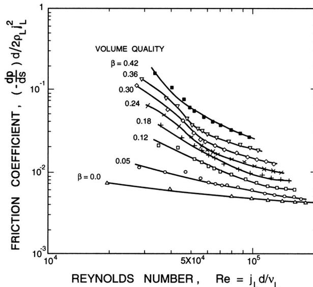
Figure 1: Typical friction coefficients (based on the liquid volumetric flux and the liquid density) plotted against Reynolds number (based on the liquid volumetric flux and the liquid viscosity) for the horizontal pipeline flow ( $d = 5.2\text{cm}$ ) of sand ( $D = 0.018\text{cm}$ ) and water at  $21^\circ\text{C}$  (Lazarus and Neilson 1978).
