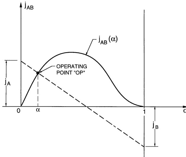
Figure 1: Basic graphical schematic or chart of the drift flux model.
