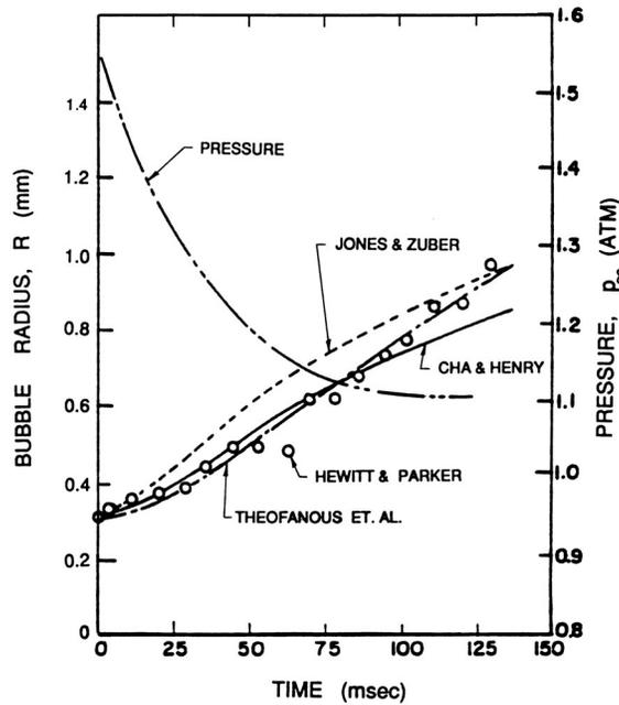
Figure 2: Data from Hewitt and Parker (1968) on the growth of a vapor bubble in liquid nitrogen (pressure/time history also shown) and comparison with the analytical treatments by Theofanous *et al.* (1969), Jones and Zuber (1978), and Cha and Henry (1981).
