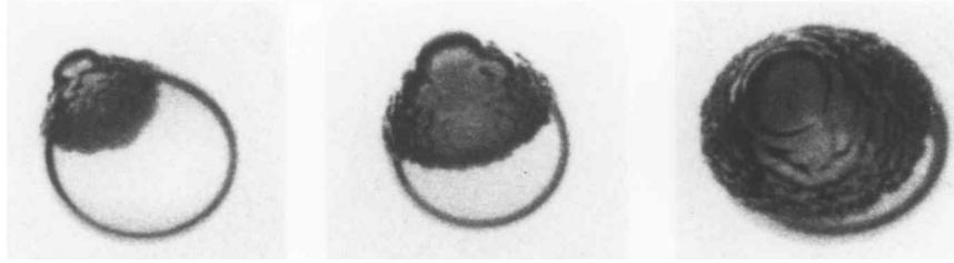
Figure 3: Typical photographs of a rapidly growing bubble in a droplet of superheated ether suspended in glycerine. The bubble is the dark, rough mass; the droplet is clear and transparent. The photographs, which are of different events, were taken 31, 44, and 58  $\mu s$  after nucleation and the droplets are approximately 2mm in diameter. Reproduced from Frost and Sturtevant (1986) with the permission of the authors.
