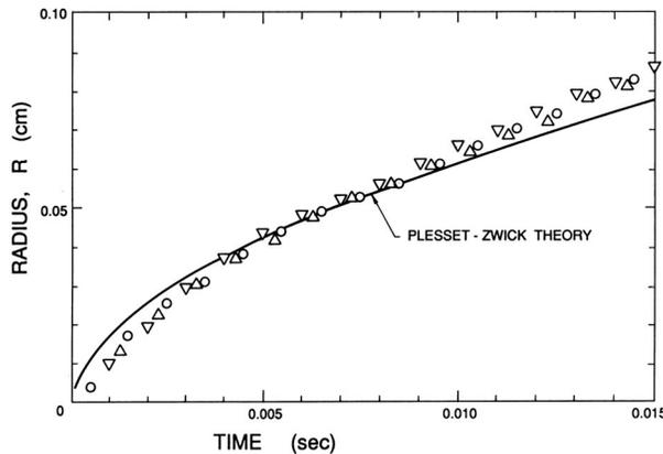
Figure 1: Experimental observations of the growth of three vapor bubbles ( $\circ$ ,  $\triangle$ ,  $\nabla$ ) in superheated water at  $103.1^\circ\text{C}$  compared with the growth expected using the Plesset-Zwicky theory (adapted from Dergarabedian 1953).
