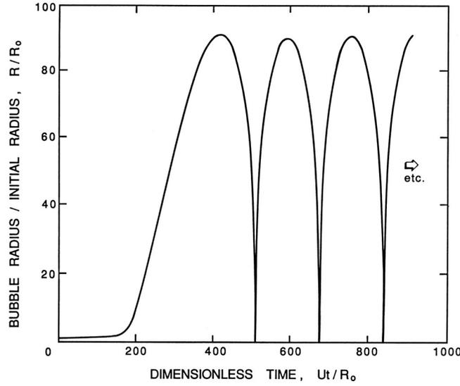
Figure 1: Typical solution of the Rayleigh-Plesset equation for a spherical bubble. The nucleus of radius,  $R_o$ , enters a low-pressure region at a dimensionless time of 0 and is convected back to the original pressure at a dimensionless time of 500. The low-pressure region is sinusoidal and symmetric about 250.
