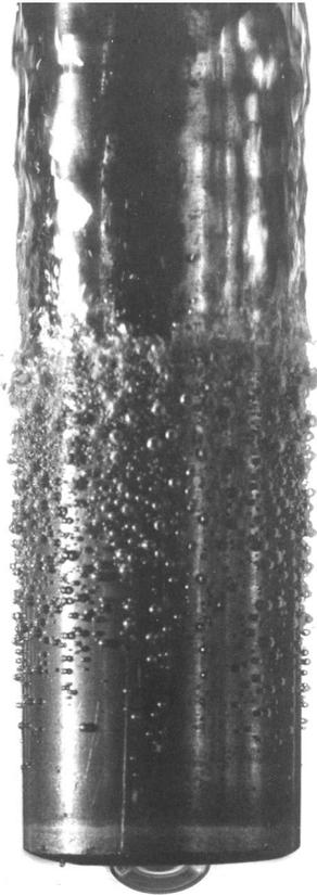
Figure 1: The evolution of convective boiling around a heated rod, reproduced from Sherman and Sabersky (1981) with permission.
