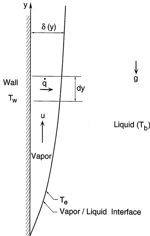
Figure 1: Sketch for the film boiling analysis.
