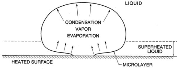
Figure 2: Sketch of nucleate boiling bubble with microlayer.
