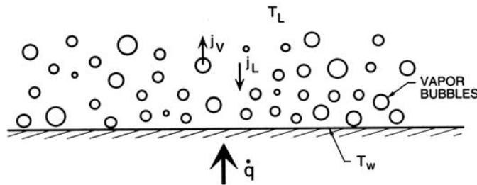
Figure 3: Nucleate boiling.
