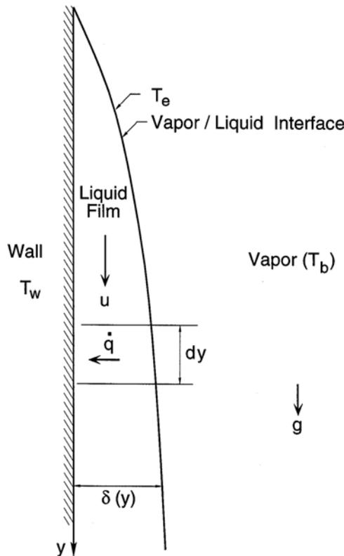
Figure 1: Sketch for the film condensation analysis.
