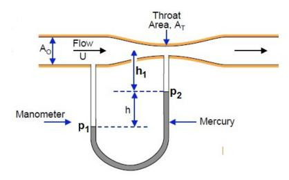
pressure taps are located upstream of the nozzle and at the throat; these are connected to a water/mercury manometer as shown. When the water is flowing through the device, the manometer levels differ by an elevation, h.
