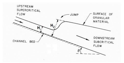
Figure 2: Notation for a granular flow hydraulic jump in an inclined chute. From Brennen et al. (1983).
