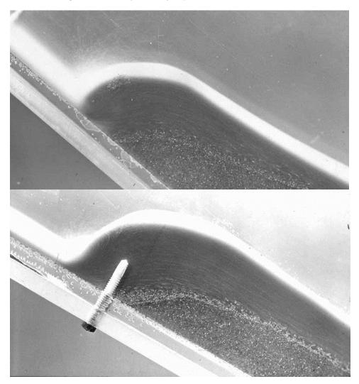
Figure 3: Examples of steady granular flow hydraulic jumps in an inclined chute. From Brennen et al. (1983).
