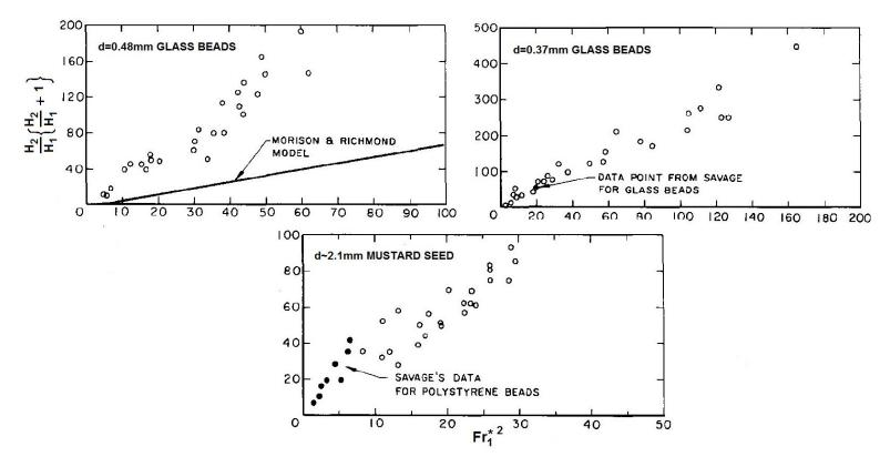
Figure 4: Experimental values of  $(H_2/H_1)[(H_2/H_1)+1]$  plotted versus  $(Fr_1^*)^2$  for granular hydraulic jumps of three granular materials and a wide range of flow rates. Adapted from Brennen *et al.* (1983).
