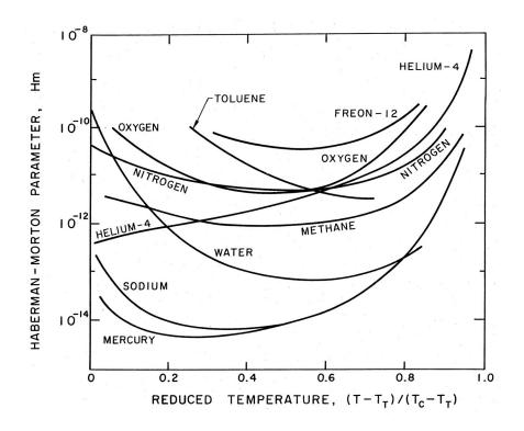
Figure 1: Values of the Haberman-Morton parameter, Hm, for various pure substances as a function of reduced temperature where  $T_T$  is the triple point temperature and  $T_C$  is the critical point temperature.
