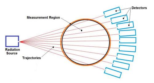
Figure 1: Schematic of a single source, tomographic arrangement deployed around a tube containing a flow.
