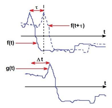
Figure 1: Cross-correlating two signals, f(t) and g(t).
