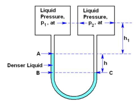
Figure 2: Basic liquid manometer for measuring liquid pressure differnces.
