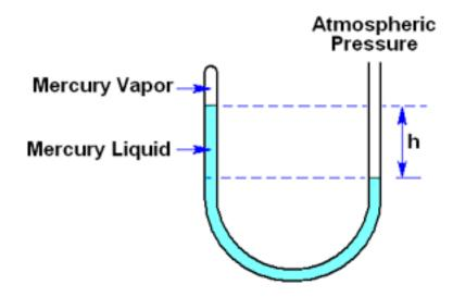
Figure 4: A mercury barometer.
