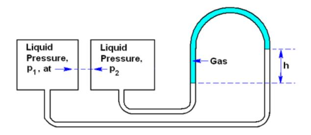
Figure 3: An inverted gas/liquid manometer.
