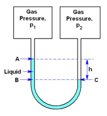
Figure 1: Basic liquid manometer for measuring gas pressure differnces.
