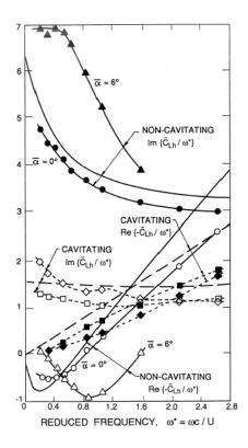
Figure 1: Fluctuating lift coefficient,  $\tilde{C}_{Lh}$ , for foils undergoing heave oscillations at a reduced frequency,  $\omega^* = \omega c/U$ . Real and imaginary parts of  $\tilde{C}_{Lh}/\omega^*$  are presented for (a) non-cavitating flow at mean incidence angles of 0° and 6° (b) cavitating data for a mean incidence of 8°, for very long choked cavities ( $\Box$ ) and for cavities 3 chords in length ( $\diamond$ ). Adapted from Acosta and DeLong (1971).
