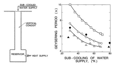
Figure 1: Left: The basic components for a geyser instability. Right: Laboratory measurements of geysering period as a function of heat supply  $(200W: \Box, 330W: \bigcirc, 400W: \diamond)$  from experiments (open symbols) and numerical simulations (solid symbols). Adapted from Tae-il *et al.* (1993).
