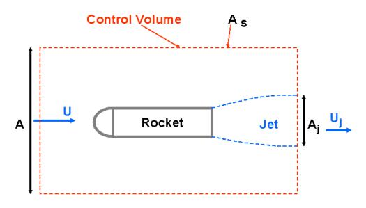
Figure 1: A cross-section through a rocket engine showing the outline of the rocket discharge (dashed blue lines) and a cylindrical control volume (dashed red lines).
