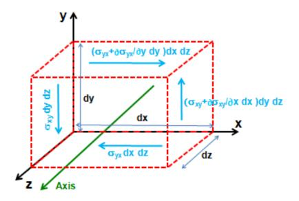
Figure 2: Forces contributing to moment about an axis parallel to z-axis.
